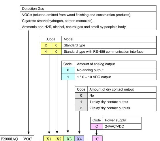
Example: F2000IAQ-VOC-2011 indicates the monitor can supply one analog output and one relay dry contact output.
