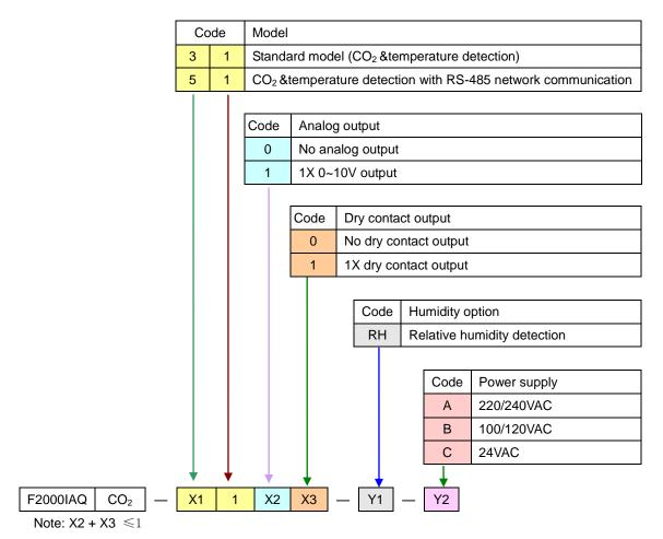
Example: F2000IAQ-CO<sub>2</sub>-3100 indicates that it is a CO<sub>2</sub> indicator with temperature detection.
